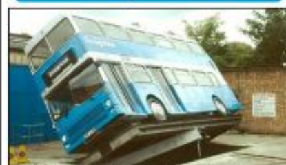
A double decker bus is being tilting to test its stability.
